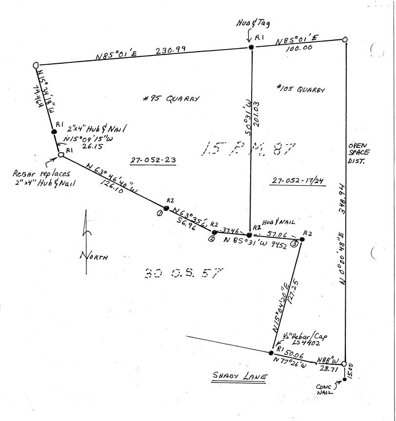
ODB = 3/4"IP LS 3887 - Pipes Reset in Concrete @ New Fence Posts - Dimensions (
