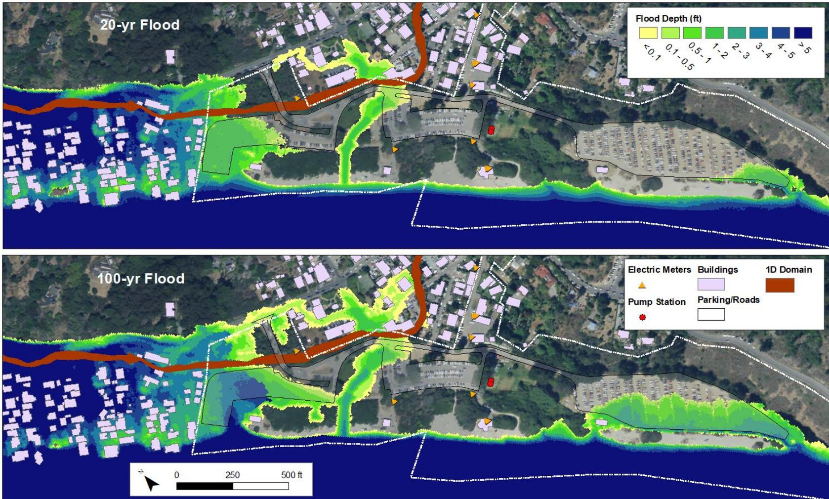
Figure 17: Combined coastal/riverine flooding for the 20-yr (top) and 100-yr recurrence interval (bottom) storm events under the 1.0 m sea level rise condition. Note that the dominant flow direction over the berm on the north edge of the north parking lot is from the GGNRA to the Calles.
