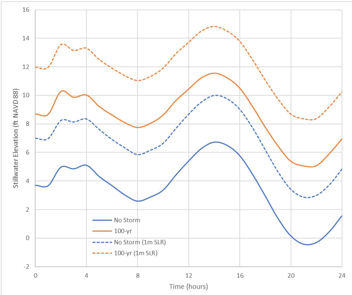
**Figure 8: Spatially-averaged stillwater elevations from CoSMoS used as boundary conditions in the hydraulic model for select storm surge and sea level rise scenarios.**
