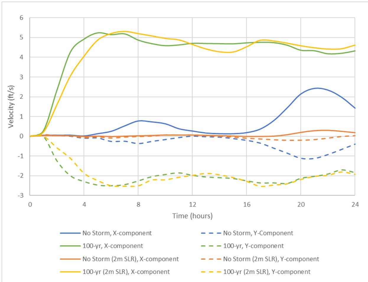
**Figure 9: Spatially-averaged velocities from CoSMoS used as boundary conditions in the hydraulic model for select storm surge and sea level rise scenarios. Note the orientation of the velocity fields is accounted for by applying x and y velocity components with the sign convention being relative to the model grid orientation.**
