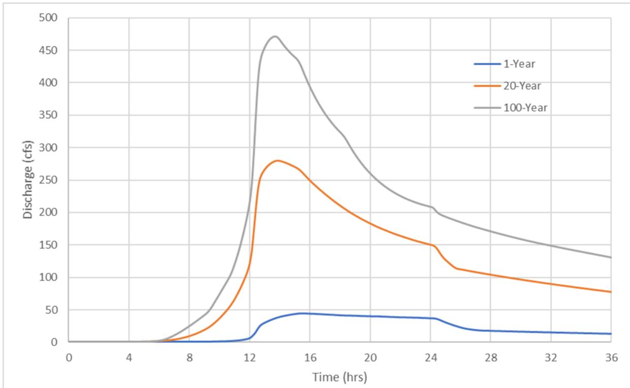
**Figure 7: Design storm hydrographs used in the hydraulic model for Easkoot Creek at Hwy 1.**
