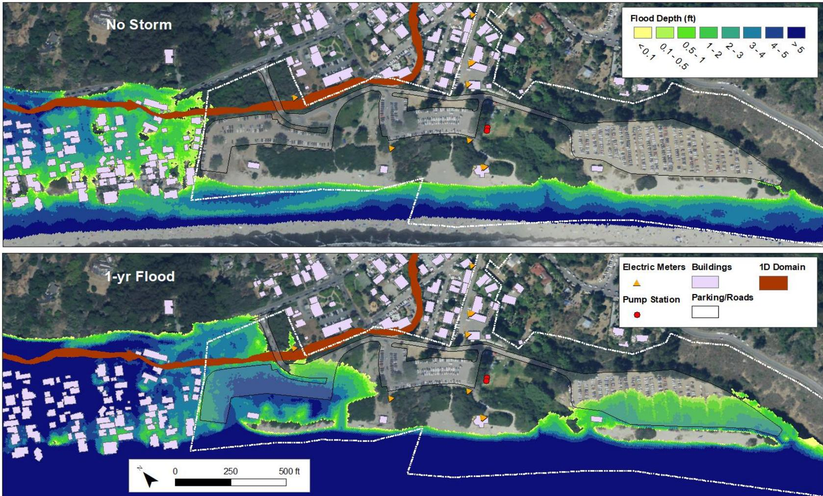
Figure 18: Combined coastal/riverine flooding for the ‘no storm’ (top) and 1-yr recurrence interval (bottom) storm events under the 2.0 m sea level rise condition. Note that the dominant flow direction over the berm on the north edge of the north parking lot is from the GNRA to the Calles.
