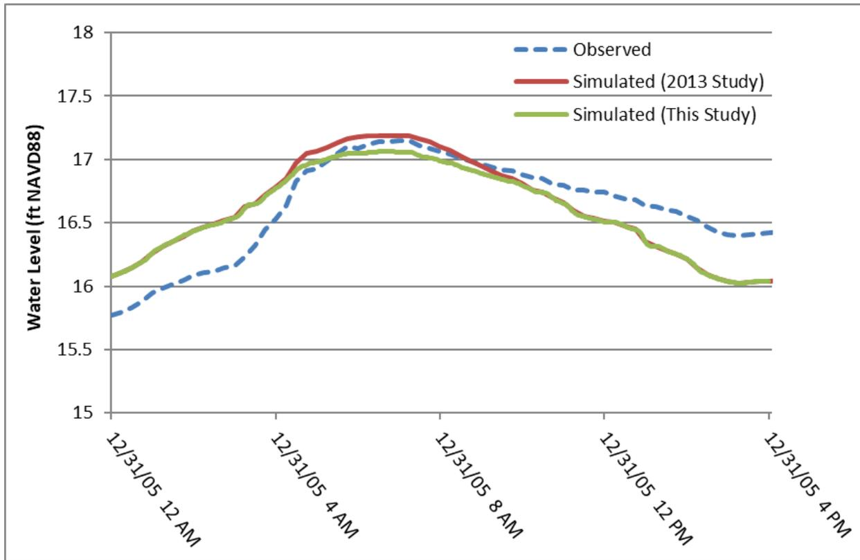
**Figure 10: Comparison between simulated and observed stages at the NPS's Easkoot Creek gauging station during the December 2005 flood.**
