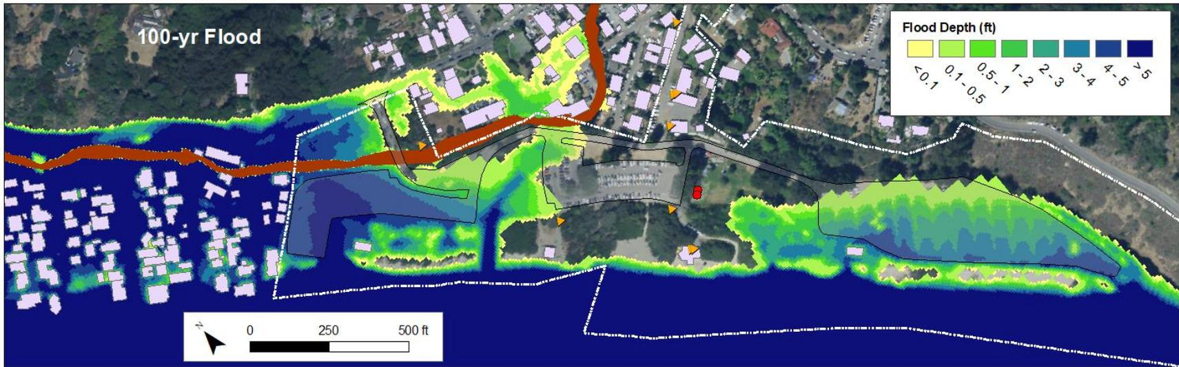
Figure 19: Combined coastal/riverine flooding for the 100-yr recurrence interval storm event under the 2.0 m sea level rise condition. Note that the dominant flow direction over the berm on the north edge of the north parking lot is from the GGNRA to the Calles.
