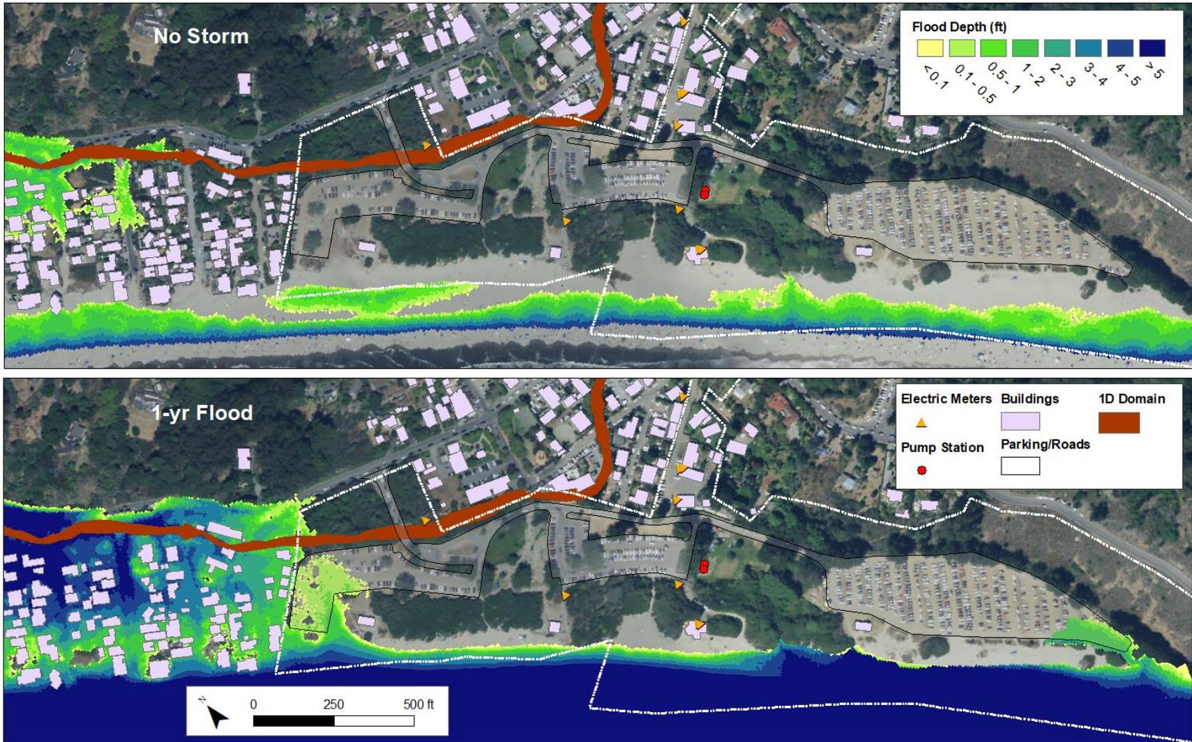
Figure 16: Combined coastal/riverine flooding for the ‘no storm’ (top) and 1-yr recurrence interval (bottom) storm events under the 1.0 m sea level rise condition.
