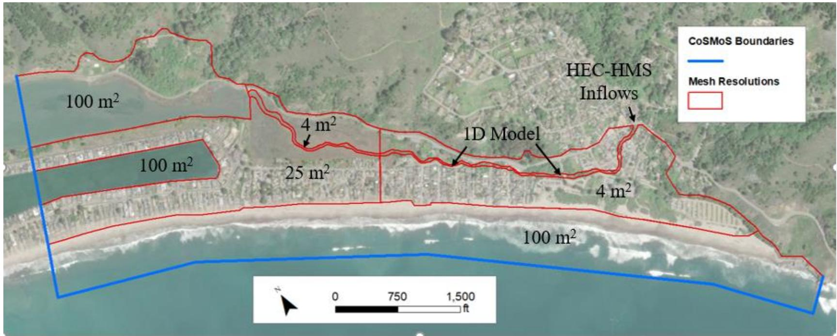
Figure 3: Extent of the hydraulic model domain, mesh resolution zones, and locations of boundary conditions applied from CoSMoS.
