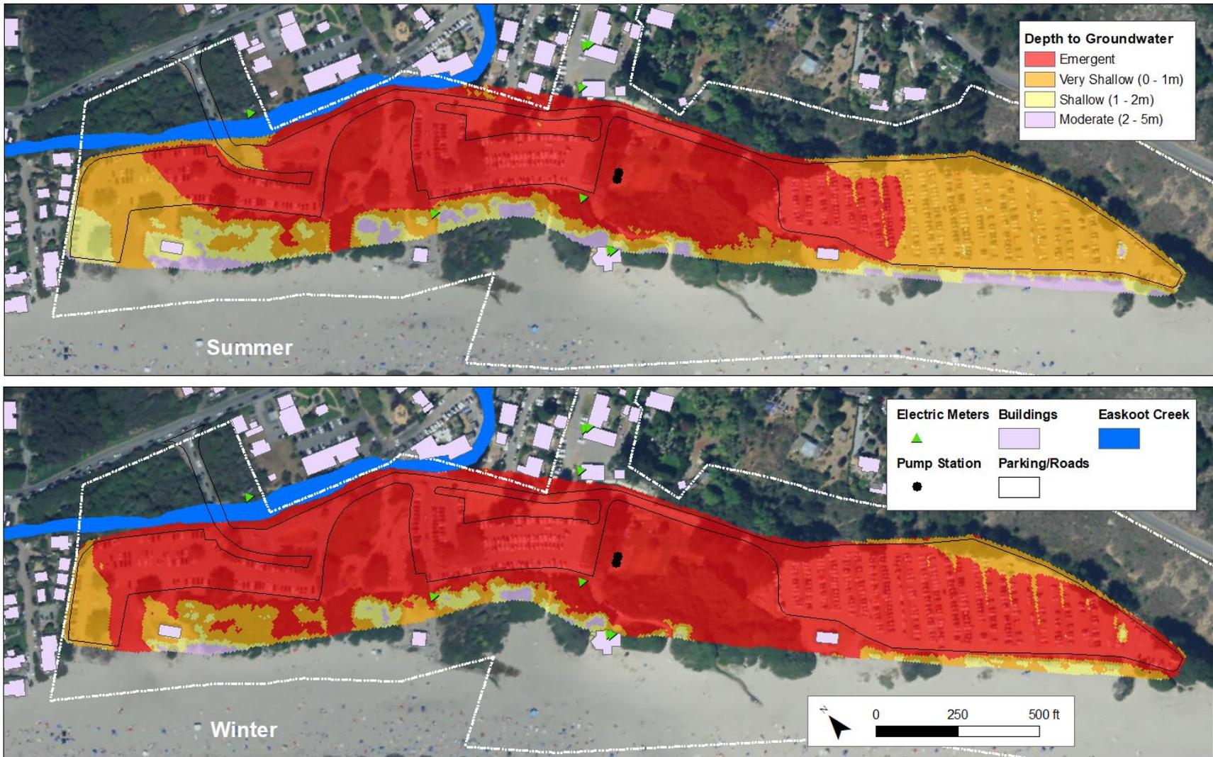
Figure 26: Estimated depths to representative summer (top) and winter (bottom) groundwater tables with 2.0 m of sea level rise assuming hydraulic conductivity of 10 m/day.
