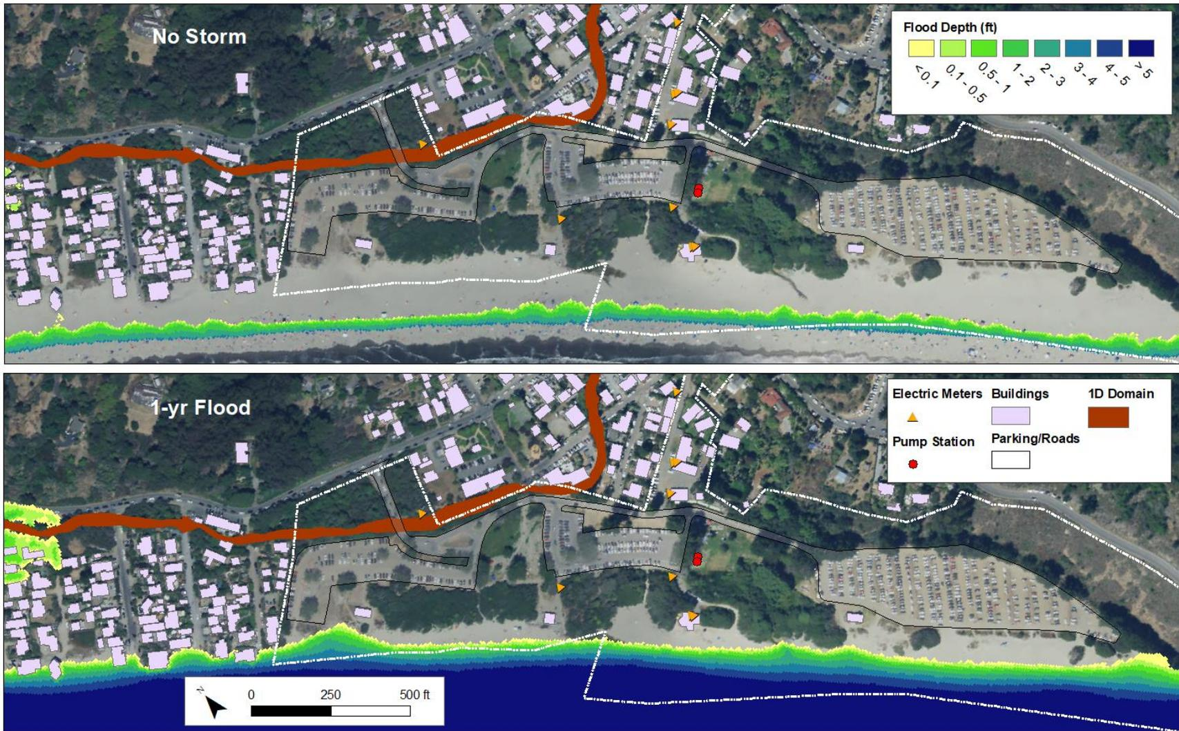
Figure 14: Combined coastal/riverine flooding for the 'no storm' (top) and 1-yr recurrence interval (bottom) storm events under the 0.5 m sea level rise condition.
