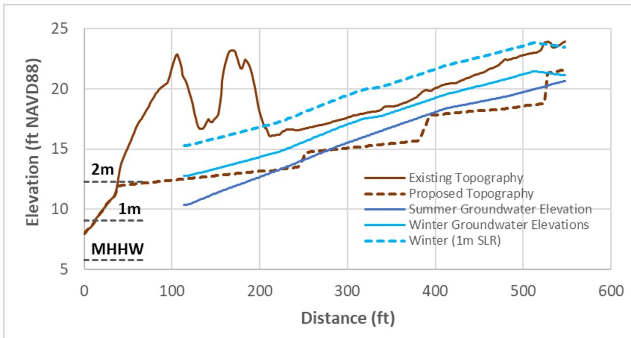
Figure 27: Longitudinal profile of the proposed bypass channel compared to water surface elevations under existing and future sea level conditions.
