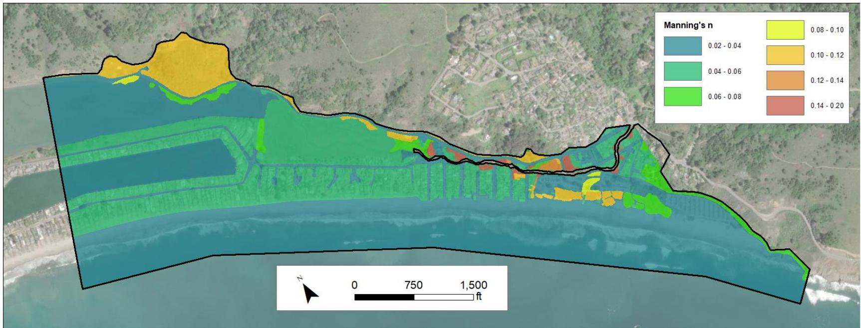
Figure 6: Manning's roughness coefficient (n) values used in 2D component of the hydraulic model.
