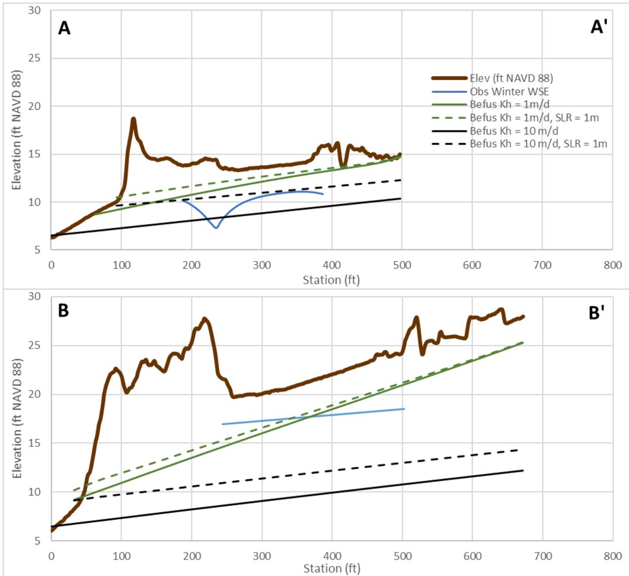
**Figure 23: Observed representative water surface elevations from NPS monitoring wells versus water surface elevations predicted by Befus et al. (2020) for various hydraulic conductivity assumptions (see Figure 21 for cross section locations).**
