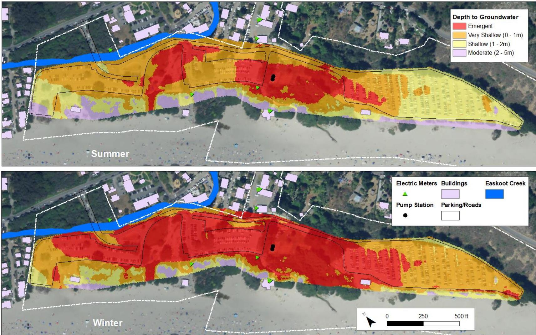
Figure 25: Estimated depths to representative summer (top) and winter (bottom) groundwater tables with 1.0 m of sea level rise assuming hydraulic conductivity of 10 m/day.
