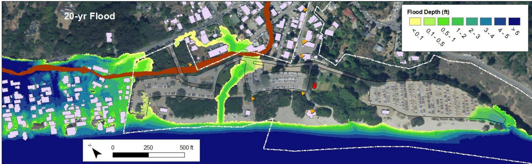
Figure 15: Combined coastal/riverine flooding for the 20-yr recurrence interval storm event under the 0.5 m sea level rise condition.
