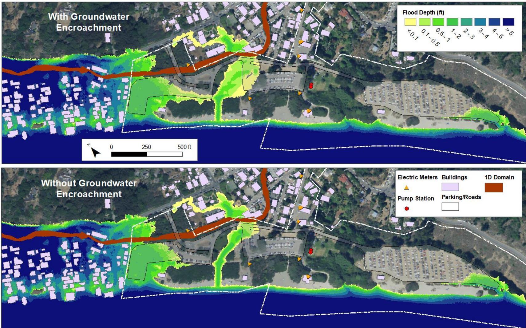
Figure 28: Combined coastal/riverine flooding for the 20-yr recurrence interval event with 1.0 m of sea level rise accounting for reduced bypass capacity due to groundwater encroachment (top) and without consideration of emergent groundwater (bottom).
