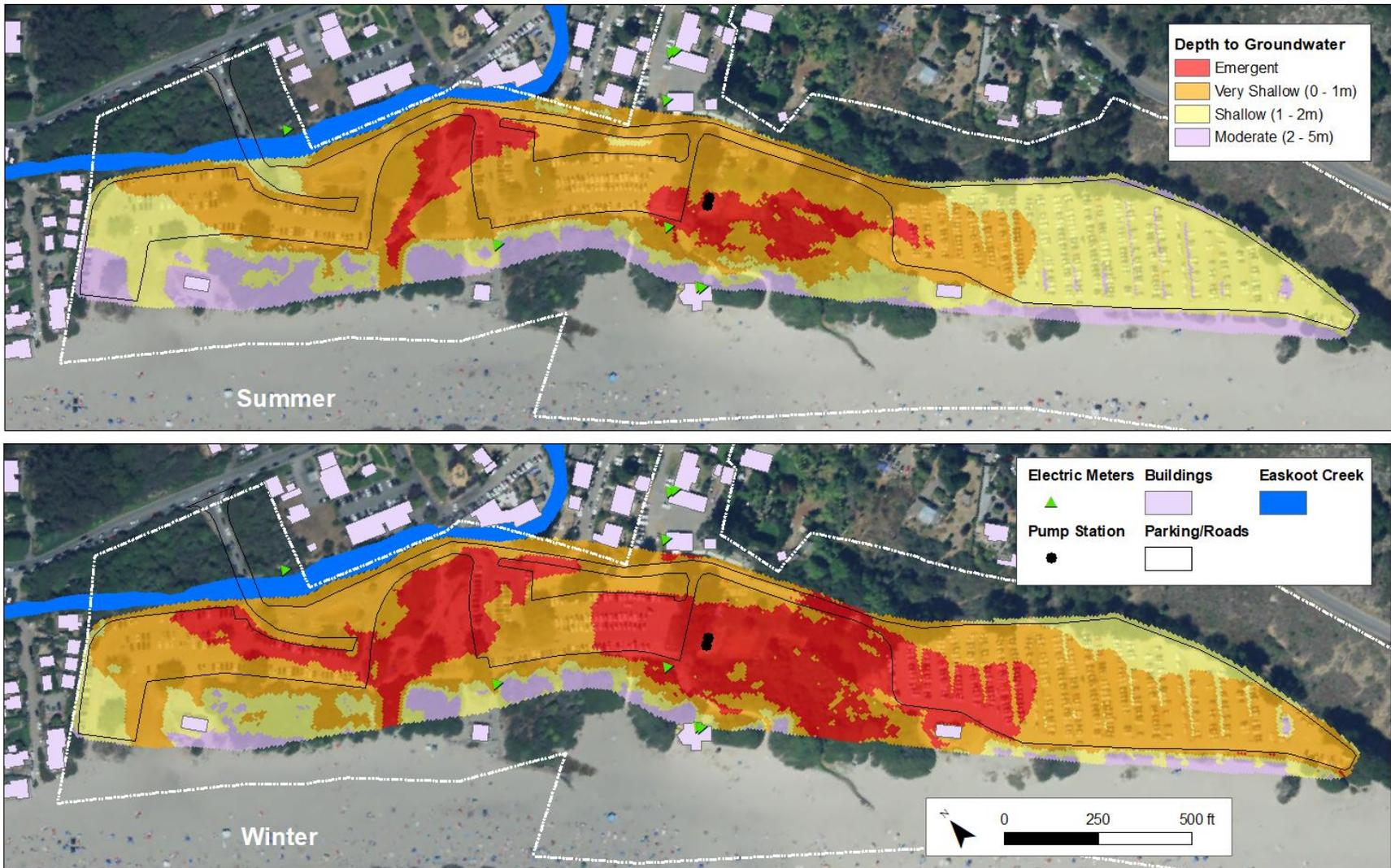
Figure 24: Estimated depths to representative summer (top) and winter (bottom) groundwater tables with 0.5 m of sea level rise assuming hydraulic conductivity of 10 m/day.
