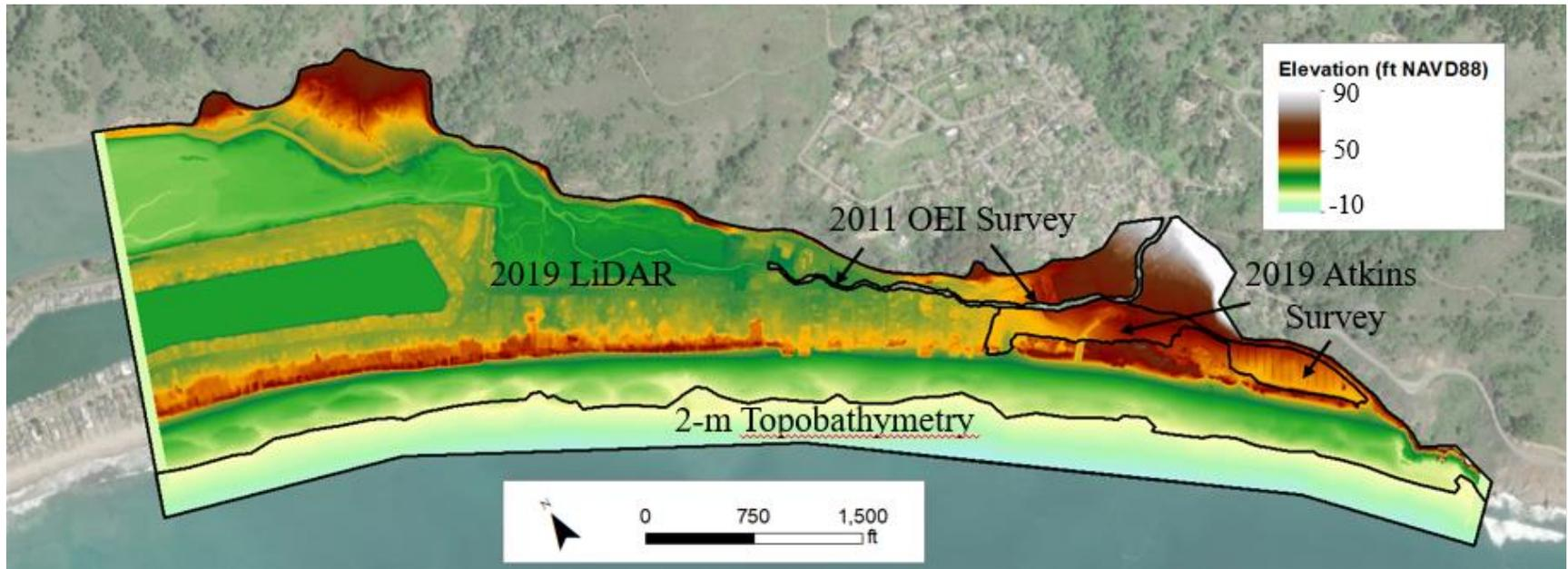
Figure 5: Digital terrain model used in the hydraulic model indicating data source areas.
