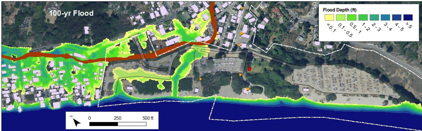
Figure 13: Combined coastal/riverine flooding for the 100-yr recurrence interval storm event under existing sea level conditions.
