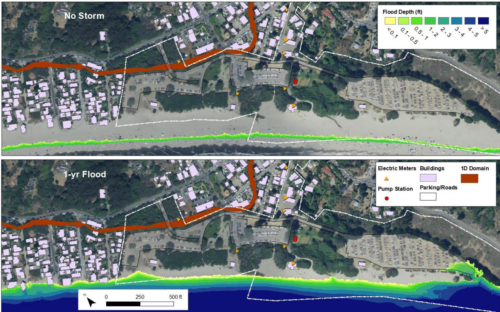
Figure 11: Combined coastal/riverine flooding for the ‘no storm’ (top) and 1-yr recurrence interval (bottom) storm events under existing sea level conditions.
