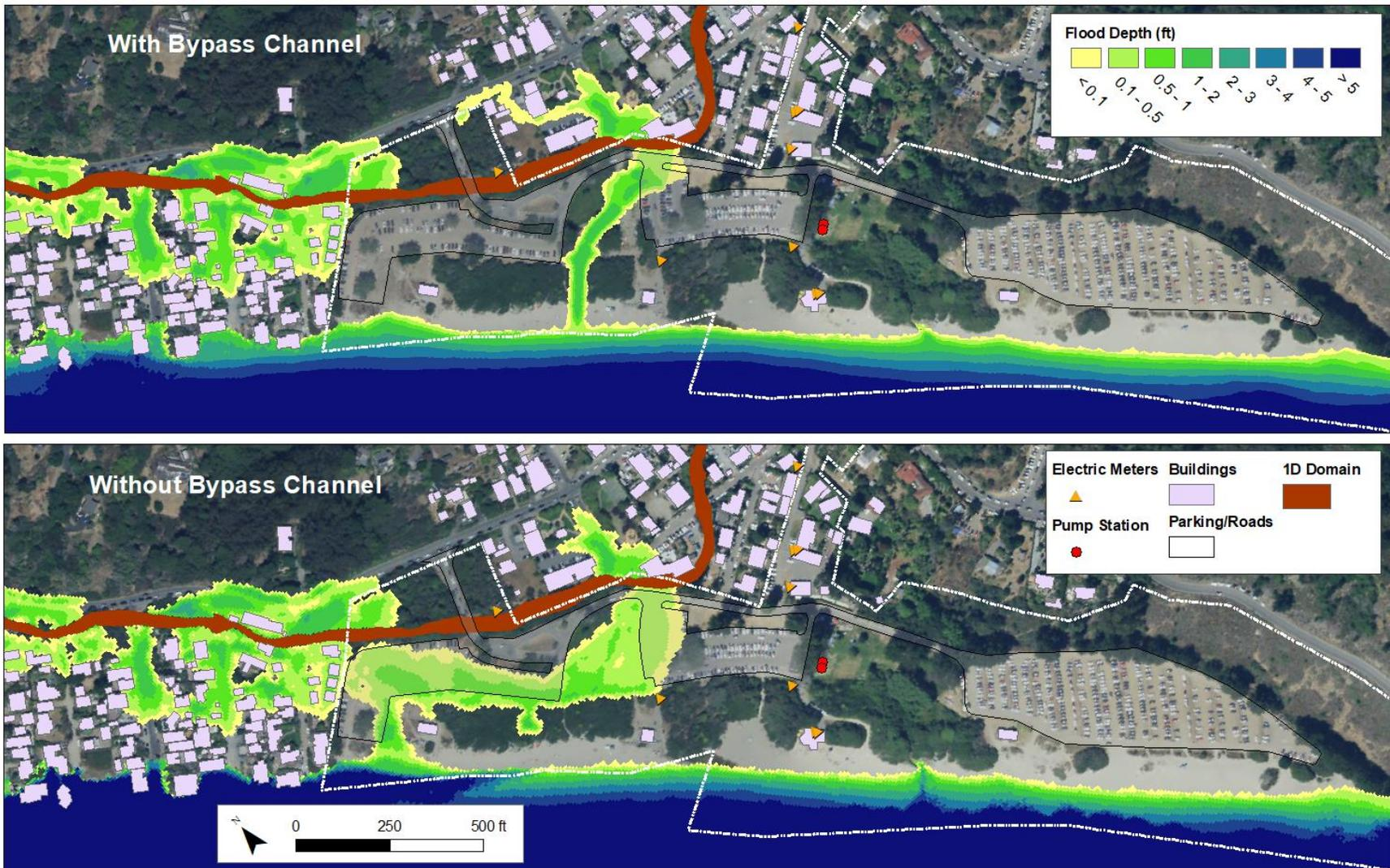
Figure 12: Combined coastal/riverine flooding for the 20-yr recurrence interval storm event under existing sea level conditions with (top) and without (bottom) the proposed bypass channel.
