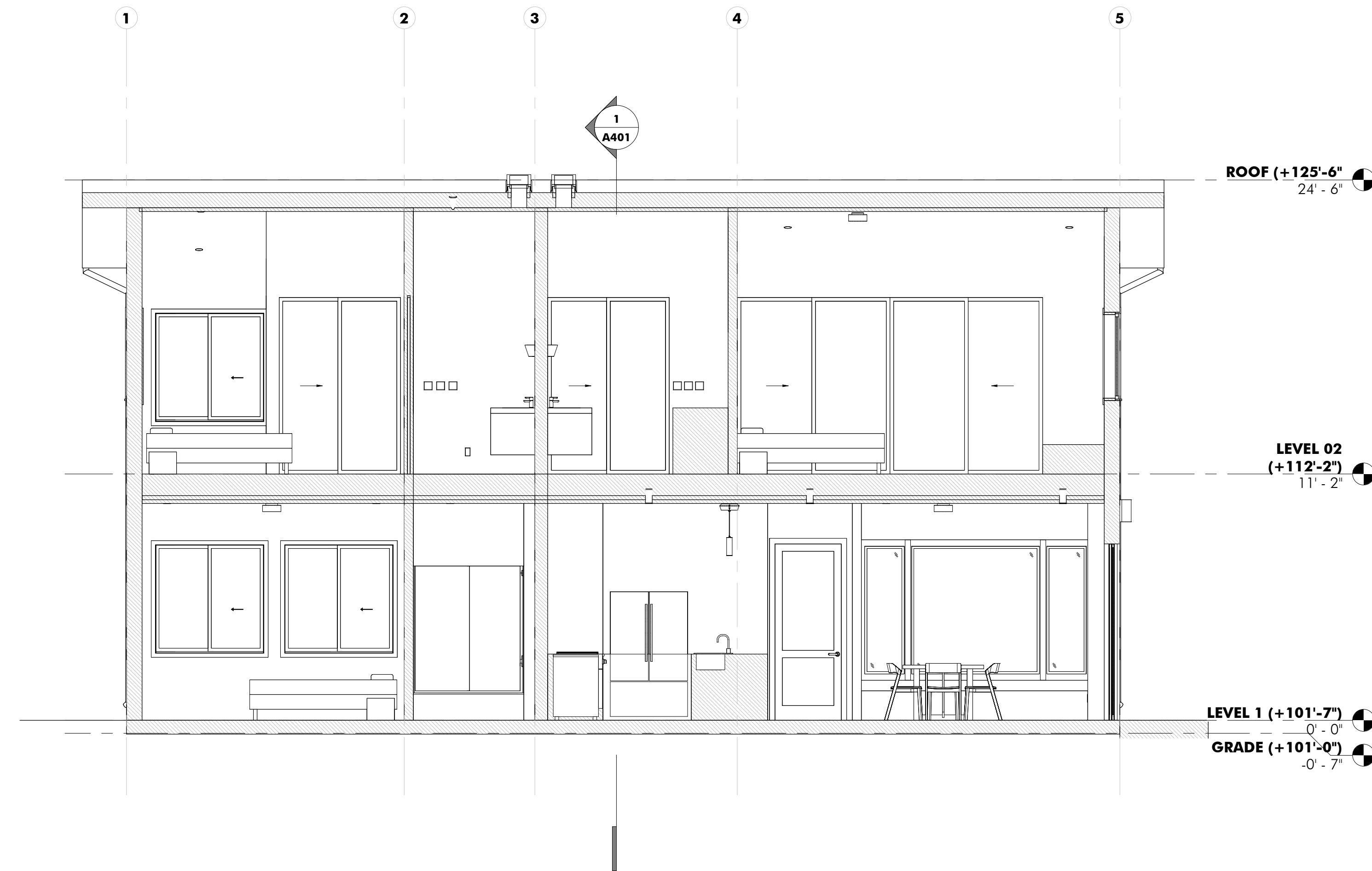
TRANSVERSE SECTION THROUGH KITCHEN 1/4" = 1'-0" 2
