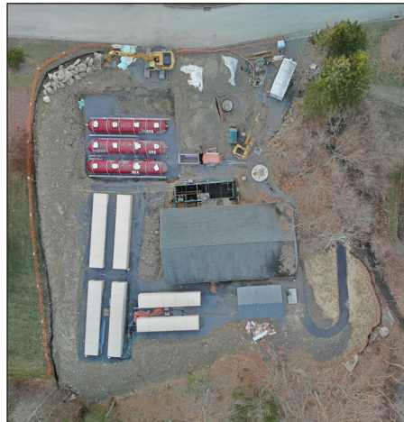
Between November and April, six AdvanTex AX-Max units were installed to replace Pinebrook's failed rotating biological contactor (RBC). The final photo on the right shows that the RBC and the building once housing it have been removed. (Photos courtesy of the Dutchess County Water and Wastewater Authority.)
