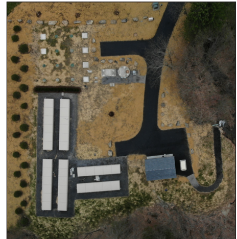
Between November and April, six AdvanTex AX-Max units were installed to replace Pinebrook's failed rotating biological contactor (RBC). The final photo on the right shows that the RBC and the building once housing it have been removed. (Photos courtesy of the Dutchess County Water and Wastewater Authority.)
